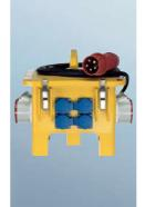
2 CEE receptacles 32A, 5p, 400V 2 CEE receptacles 16A, 5p, 400V 2 MCB's 16A, 3p, C 4 SCHUKO® receptacles 16A, 230V 2 MCB's 16A, 1p, B 1 RCD 40A, 4p, I<sub>AN</sub> = 0.03A Feeder cable 3 m H07RN-F5G4 with CEE plug 32A, 5p, 400V
