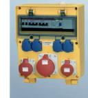
1 MCB 32A, 3p, C 1 CEE receptacle 16A, 5p, 400V 1 MCB 16A, 3p, C 4 SCHUKO® receptacles 16A, 230V 2 MCB's 16A, 1p, B 1 RCD  $\stackrel{\frown}{\boxtimes}$  63A, 4p,  $I_{\Delta N} = 0.03A$ preferably with connection for 2 cables of up to 5 x 25 mm<sup>2</sup>
