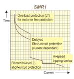
A trip unit designed to offer a overload (LT) and short-circuit protection (ST). The overload protection is adjustable from 0.4 to 1 x the chosen rating and has two protection bands (LTD), one for line protection and one for motor protection (class
