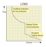
This trip unit offers overload and short-circuit protection.
