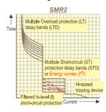
A trip unit designed to offer a overload (LT) and short-circuit protection (ST). The overload protection is adjustable from 0.4 to 1 x the chosen rating and has multiple protection bands (LTD). The short-circuit protection (ST) is adjustable from 2
