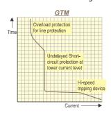
A trip unit de signed to offer overload and short-circuit protection. The overload protection is adjustable from 0.8 to 1 x the chosen rating whilst the short-circuit protection is set at about 4 x the chosen rating (FD frame) or adjustable from 2.5 to
