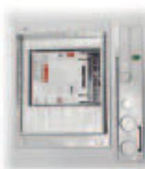
The F-WM kit allows the operating panel of a Record Plus Electrical operator and the draw-out euchenon to be accessed on the door front. The kit includes an extension frame, a doorflange and the through door euchenon with it's locking and position indication features.
