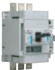
The draw-out device is supplied as a complete entity including a mobile and fixed part allowing the conversion of a standard fixed front connection breaker to a draw-out type. It includes a racking handle and can be used behind or through door without any additional accessories. The draw-out device is available with front or Rear connections.
