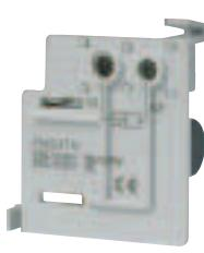
When the breaker is in the ON position and the shunt trip is activated the breaker will trip and its contacts will open. The device can be constantly activated at its nominal voltage allowing it to be used as a lock out coil. The connection clamps are marked C1 and C2. Switches, relay contacts and push buttons are used to operate the shunt release.
