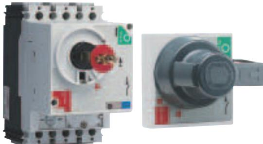
A handle and escutcheon is mounted on the door or panel front and connected to the breaker by an elongation shaft that goes into an adaptor box directly installed onto the breaker front. The design allows for a total depth of up to 350 mm (from the back of the breaker mounted behind the door or panel and the door front).
